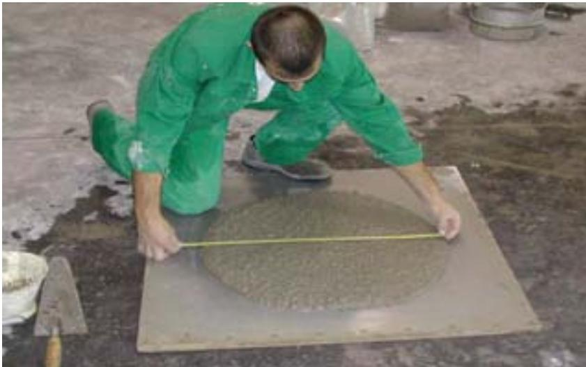
**Figure 9.1. Slump-flow test**
