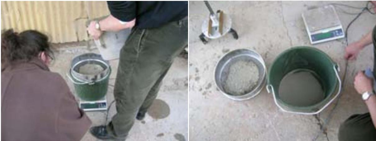
Figure 8.4 Sieve segregation resistance test
