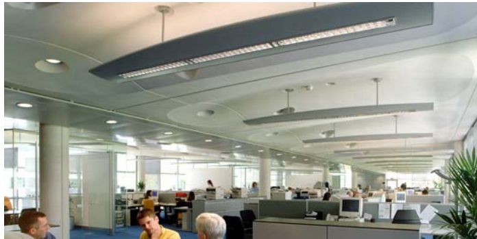
Figure 1b: A comfortable office environment is provided by using concrete's thermal mass to full advantage: Toyota Headquarters, UK. (Courtesy of the Concrete Society, UK)
